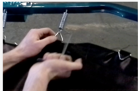
C. Hook the loose end of the spring through the metal triangle on the net.
