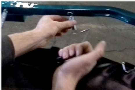
A. Grab a spring in one hand and the Net Assembly tool in your other hand.
