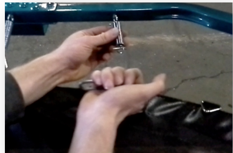
B. Hook the Net Assembly Tool through the loose end of the spring.
