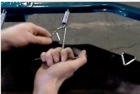
C. Pull with the Net Assembly Tool to stretch the spring toward the net.
